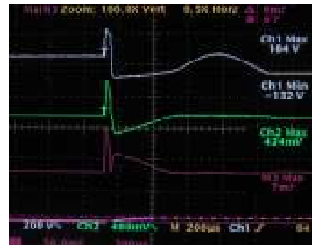
Surge-testing: Measuring and calculating residual surge energy at output side of signal SEAT after combination waves 1.2x50 \mu s, 2.5 kV ;8x20 \mu s 1.25kA are coupled to input side of signal SEAT .
