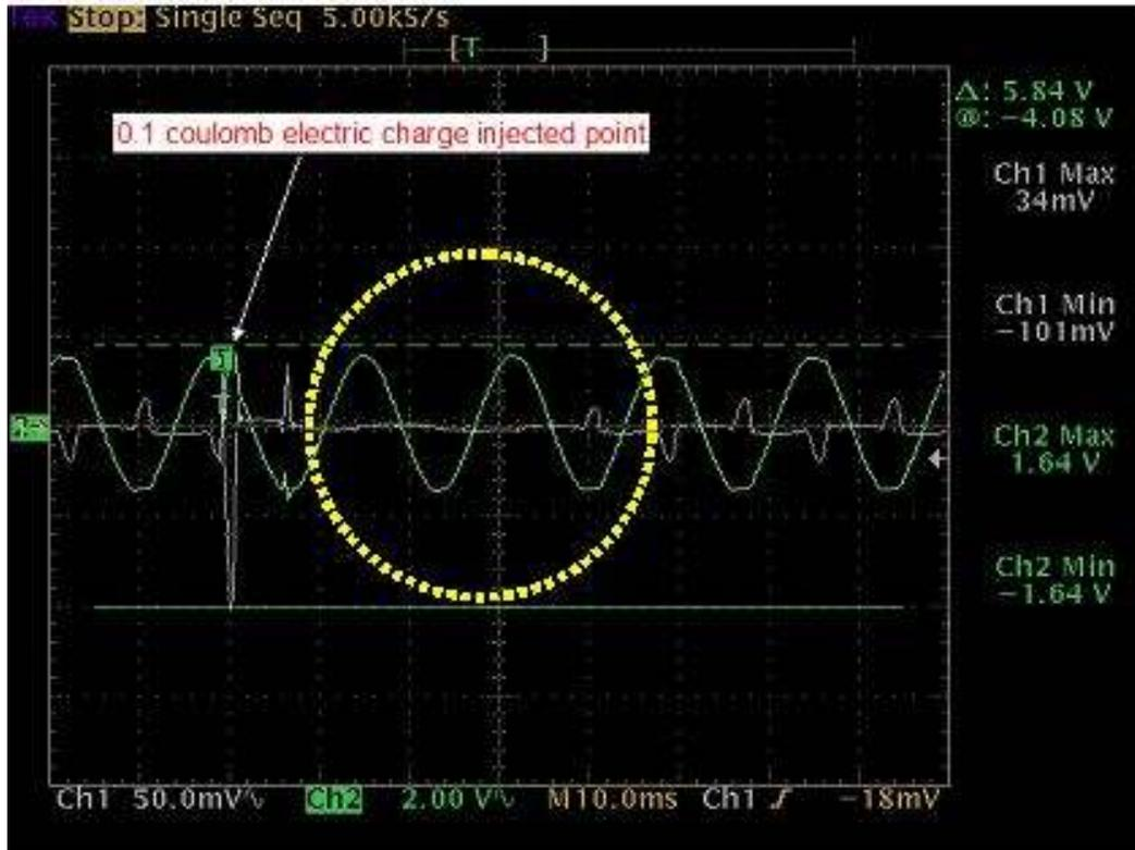
Due to surge energy being converted into voltage, converted voltage overlaps with AC power waveform within 2 cycles (circled by yellow dotted line)
